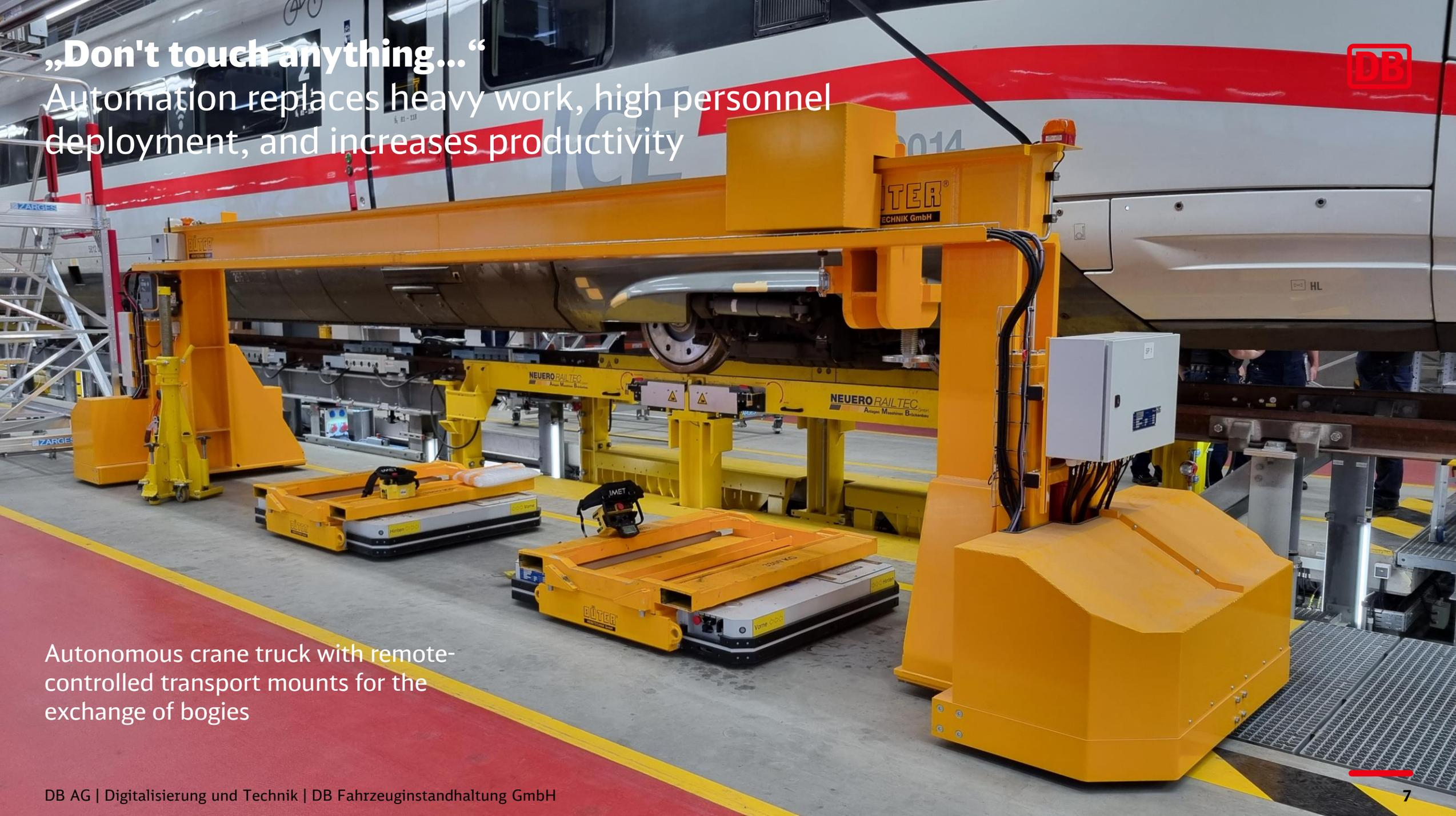
Autonomous crane truck with remote-controlled transport mounts for the exchange of bogies
