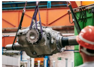
Gearbox housing BR29x using Rapid Casting
